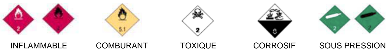
Figure 7. Losanges de danger
